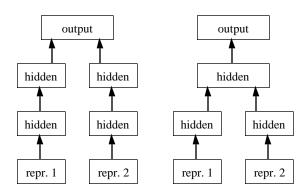
Figure 7. Two architectures for combining different input representations in a classifier net. Each box represents about 100 neuron units, and each heavy arrow corresponds to about 10,000 weights. The more separated architecture (left) seems to work better; the alternative that combines information at a hidden layer (right) is smaller but "too powerful."
