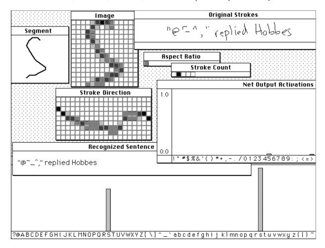
Figure 9. Some of the kinds of windows available in our research recognizer. The net output window is wrapped to fit all 94 printable-ASCII characters in the figure. In the example shown, an intended *hyphen* has been mis-classified as *underscore*.
